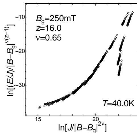
Fig. 2. (a) Observed  $E$ - $J$  characteristics at various magnetic fields and at  $T = 40$  K and (b) their scaled result.
