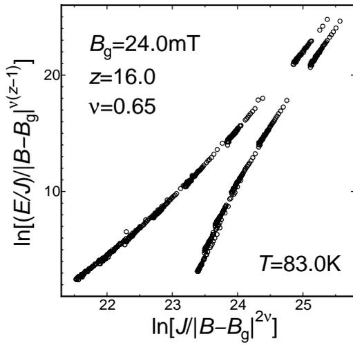
Fig. 3. (a) Observed  $E$ - $J$  characteristics at various magnetic fields and at  $T = 83$  K and (b) their scaled result.
